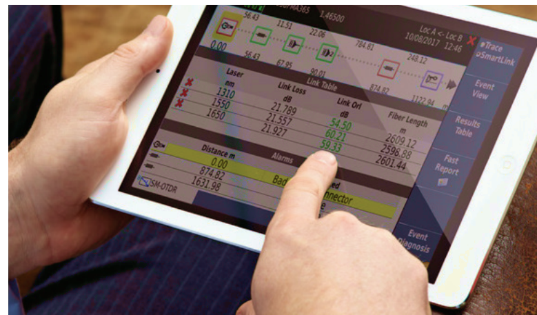
The lead engineer can view the user interface of a new tech's OTDR remotely from his office chair
