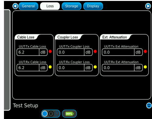
Fig. 12 Test Setup Loss Tab Screen
